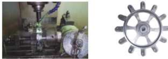
Fig. 8. The processing of positioning slots
