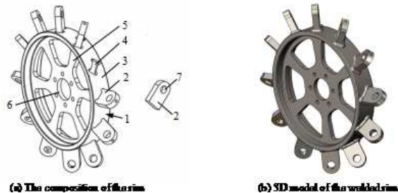
Fig. 7. The structure of the wheel rim
