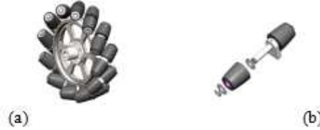
Fig. 9. Assembly of the Mecanum wheel
